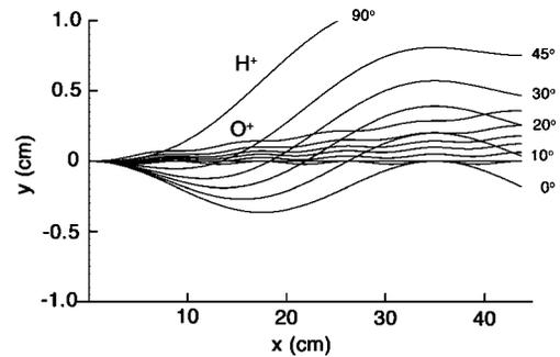
FIG. 2. Plot of the calculated path of  $H^+$  and  $O^+$  ions with energies/charge of  $1 \text{ keV}$  through a parallel-plate analyzer segment with no dc voltage applied but with a peak  $5 \text{ MHz}$  rf voltage of  $150 \text{ V}$  across a  $4 \text{ mm}$  analyzer gap. The phases of the rf voltage when the ions enter the analyzer are noted on the  $H^+$  curves.
