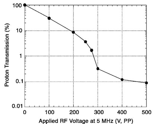
FIG. 5. Results of the laboratory test showing transmission factor of protons as a function of the peak-to-peak voltage of the rf deflection potential.
